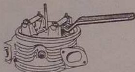
Compression des ressorts de soupapes
